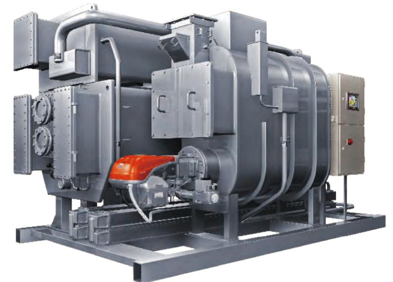
H2-type direct fired lithium bromide absorption chiller/heater is a kind of large-size industrial facility to supply cool or heat with gas (natural gas, city gas, or LPG) or oil (diesel oil) as the driving energy and lithium bromide solution as the absorbent and water as refrigerant.
